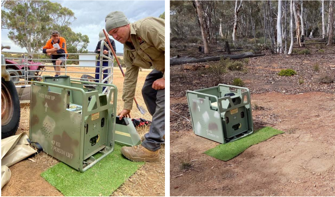
Figure 2. (Left) Felixer set up near farm sheds with flat ground in front of the unit for accurate measurements of passing animals and (right) in native vegetation. Artificial grass helped prevent mud or sand splashing sensors during rain events.
