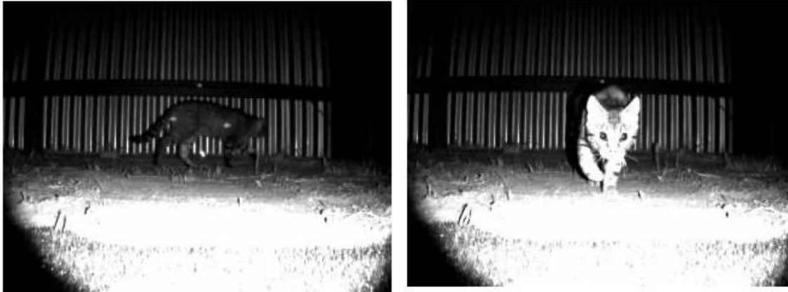
Figure 6. Angle of approach by a feral cat influences whether or not it satisfies the criteria to be moving as expected for a feral cat, and therefore whether the Felixer unit considers it to be a target. Left: target photo, right: non-target photo.
