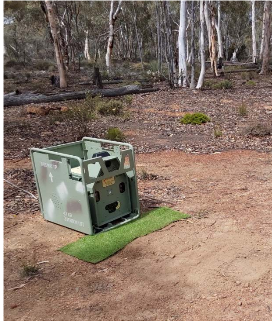
Figure 2. (Left) Felixer set up near farm sheds with flat ground in front of the unit for accurate measurements of passing animals and (right) in native vegetation. Artificial grass helped prevent mud or sand splashing sensors during rain events.
