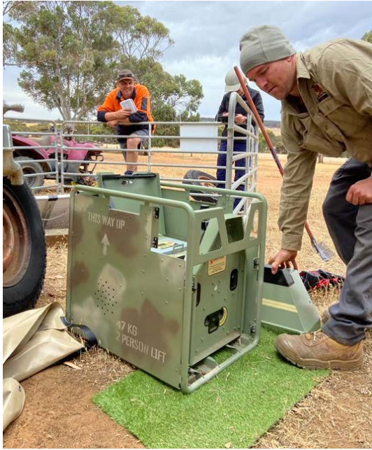
Figure 2. (Left) Felixer set up near farm sheds with flat ground in front of the unit for accurate measurements of passing animals and (right) in native vegetation. Artificial grass helped prevent mud or sand splashing sensors during rain events.
