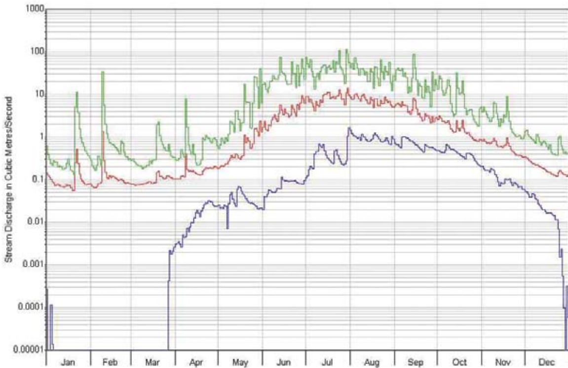
Figure 15b: Log flow chart for the Serpentine River at the primary LMU site (limit of tidal flushing) Station 614030. Daily maximum (green), daily minimum (blue) and daily mean (red). Period of record 21/02/1979 to 13/06/2005 (courtesy Department of Water).
