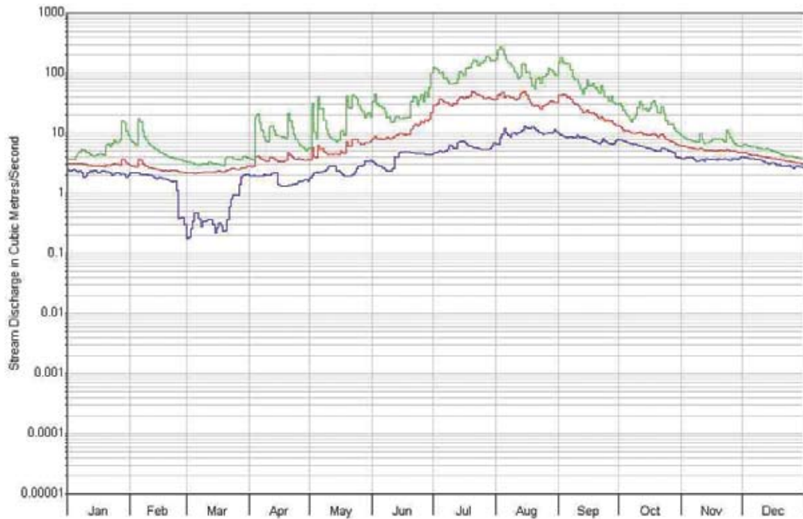
Figure 16b: Log flow chart for the Murray River at the primary LMU site (limit of tidal flushing) Station 614065. Daily maximum (green), daily minimum (blue) and daily mean (red). Period of record 23/10/1991 to 09/06/2005 (courtesy Department of Water).
