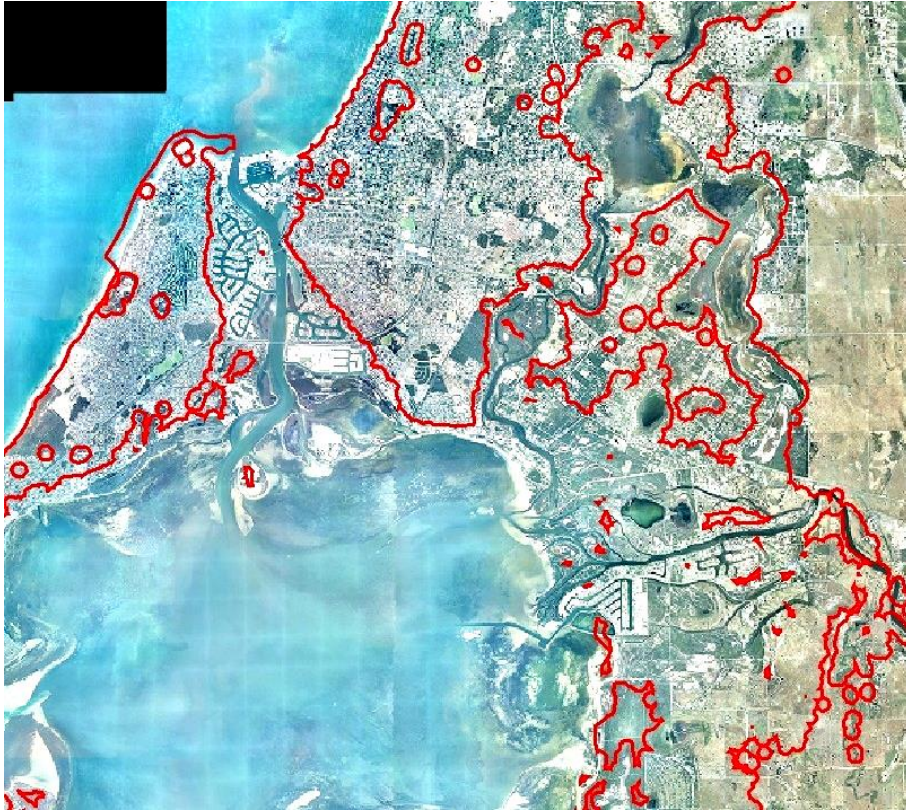
Figure 25: The interpolation contour for a 1m sea level rise coupled with an approximate lateral buffer zone of 100m overlaid on aerial photography that has already been incorporated into the PHCC DSS. This line indicates possible infrastructure and natural resources that would be directly affected by such a change in the Peel Region.
